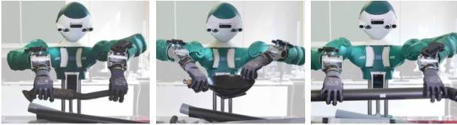
Fig. 9: The humanoid robot ARMAR-6 grasping and carrying multiple objects (exhaust, pan, and pipe) bimanually.
