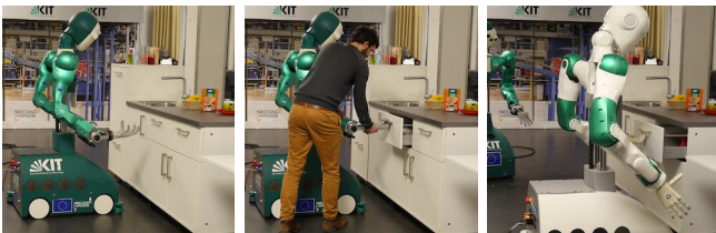
Fig. 10: Transfer of drawer opening skill learned through kinesthetic learning from ARMAR-6 to ARMAR-DE.
