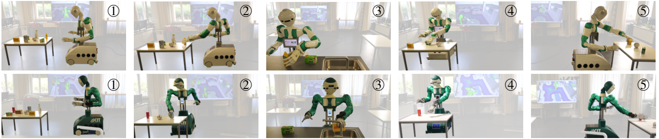
Fig. 7: Table-clearing of known and unknown objects with ARMAR-DE and ARMAR-6. ① Initial setup, ② grasping of known objects, ③ placing of known objects, ④ grasping of unknown objects, and ⑤ placing of unknown objects.
